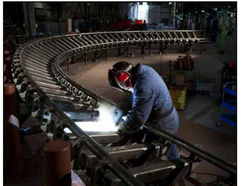
Among its projects for The Disneyland Resort, Dynamic Structures completed an extensive refurbishment of the property's monorail trains (top) and a full track replacement and systems upgrade inside Disneyland's Space Mountain (right). The company's specialized, high-precision box girder method of coaster track construction (above) allows for maximum geometric flexibility and durability. COURTESY DYNAMIC STRUCTURES
