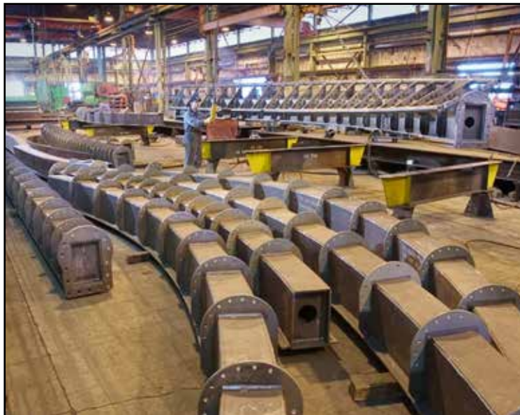
Among its projects for The Disneyland Resort, Dynamic Structures completed an extensive refurbishment of the property's monorail trains (top) and a full track replacement and systems upgrade inside Disneyland's Space Mountain (right). The company's specialized, high-precision box girder method of coaster track construction (above) allows for maximum geometric flexibility and durability. COURTESY DYNAMIC STRUCTURES
