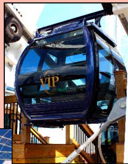
The SkyWheel at Myrtle Beach Landing — a new Chance Morgan R60 Giant Wheel — debuted this spring. The 187-foot-tall ride features 42 glass-enclosed, temperature-controlled gondolas that hold up to six passengers each. AT/SCOTT RUTHERFORD
