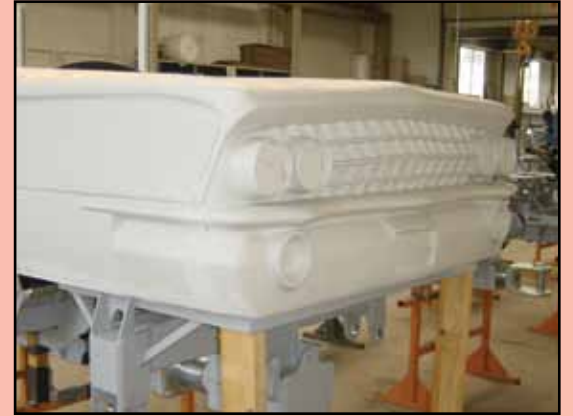
A full size mock up of the coaster vehicle, above left, was done in stages at the Gerstlauer factory, before a mold could be cast. This produced the finished themed design in fiberglass, shown above right. COURTESY GERSTLAUER
