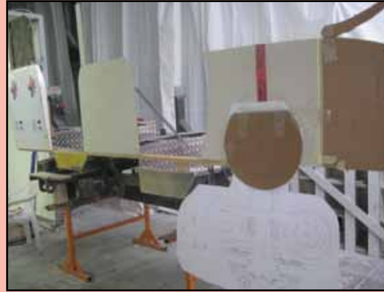
A full size mock up of the coaster vehicle, above left, was done in stages at the Gerstlauer factory, before a mold could be cast. This produced the finished themed design in fiberglass, shown above right. COURTESY GERSTLAUER
