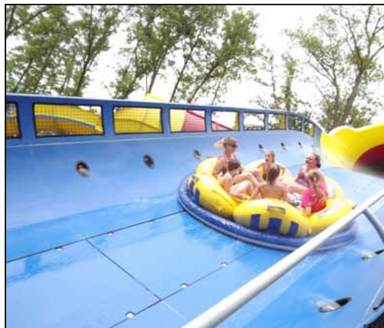
ProSlide used Holiday World's natural terrain in the design of Mammoth. The HydroMagnetic water coaster features 100 LIM's to power the rafts through the course providing a capacity of 1,000 pph. COURTESY PROSLIDE
