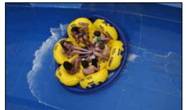
Holiday World & Splashin' Safari's new Mammoth HydroMagnetic water coaster from ProSlide is a record setter. The $9 million ride is the world's longest such ride at 1,763 feet, and uses 100 LIM's to blast the six-passenger rafts through the course. COURTESY PROSLIDE
