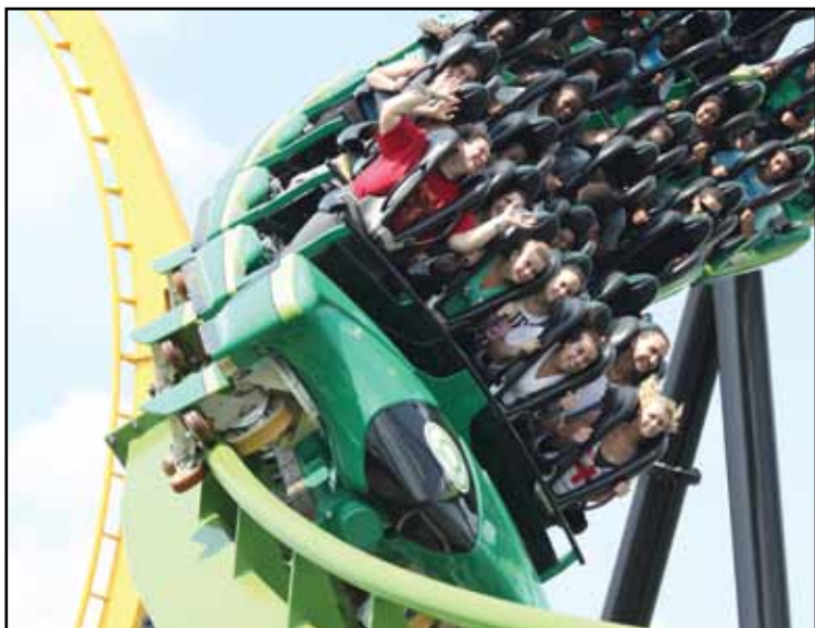
Six Flags Great Adventure's new-for-2011 major attraction is Green Lantern, a B&M stand-up coaster relocated from now-closed Kentucky Kingdom. The 154-foot-tall ride features a 121-foot-tall loop, a 103-foot dive loop, a 72-foot inclined loop and double corkscrew. AT/GARY SLADE
