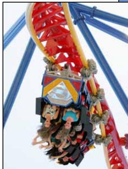
**Superman's 12-passenger train negotiates its course at a top speed of 62 mph, carrying riders through a heartline roll 150 feet above the ground and braking twice for added drama before diving into its most contorted elements.**
