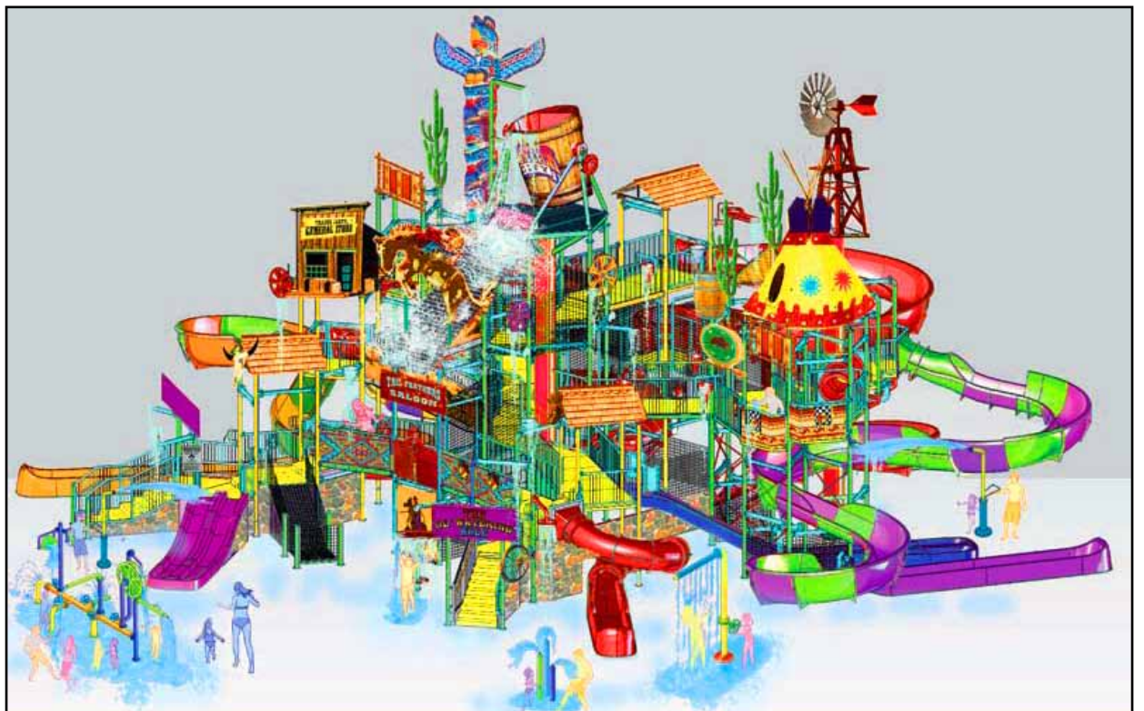
Frontier City has partnered with Canada's WhiteWater West to produce Wild West Water Works, a custom themed AquaPlay RainFortress, for the 2012 season. The 52-foot-high interactive play structure will feature a 1,000-gallon tipping barrel, 200 interactive play elements and eight waterslides. COURTESY WHITEWATER
