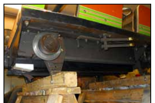
Waldameer Park has added magnetic braking into the curving brake run/station of the park's historic Comet coaster, a first for Velocity Magnetics. COURTESY WALDAMEER
